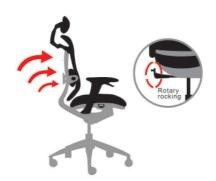
2.Pull the knob on the lower right of the seat; turn clockwise to increase tension, counterclockwise to decrease tension.
