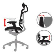
Lifting up and pushing down on the armrest will adjust the height and the arm pads pivot.
