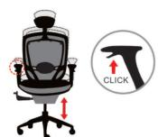
1.Pressing up on the lever under the right armrest will adjust the height of the seat. The weight of the body will make the seat lower when gripping the lever and release it; the seat will stop at the desired position. Gripping the lever when there is no weight on the seat makes it rise.
